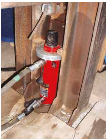
HD cylinders can be used in pushing and pulling applications. In this photo, we see a HD2506 HD cylinder set up for a pull application using a plunger clevis cylinder accessory
