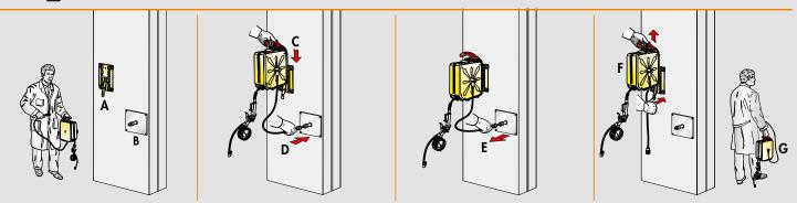
Quick Hooking and quick Release of the hose reel at every work point. Bayonet bracket easy wall-mounting (A), quick connection to compressed-air system (B), quick connection of hose-reel to wall bracket (C), quick connection of hose reel to compressed-air system (D). Release: quick release from compressed-air system (E), quick release of hose-reel from wall bracket (F), easy to carry handle reduced weight (G).
