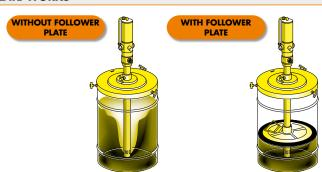
The atmospheric pressure at sea-level is 1 bar, equivalent to approx. 1 kg per cm<sup>2</sup>. When the pump sucks the grease from the container, a vacuum is created under the follower plate and, at the same time, depending on the width of its surface, a pressure from 370 kg to 2000 kg is created above it.
